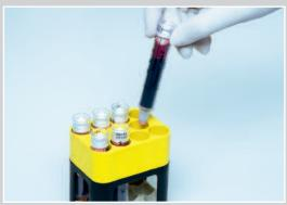
Unlike the conventional blood collection tube the Primavette® sepa is set into the centrifuge rack headfirst. In order to guarantee an ideal centrifugation, it is essential to use special centrifuge inserts (available from KABE LABORTECHNIK). The centrifugation in centrifuges with 90° swing-bucket rotors is recommended.
